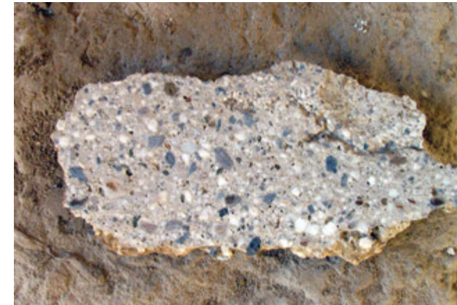
9. A section of gypsum plasterwork containing a large amount of gravel.
