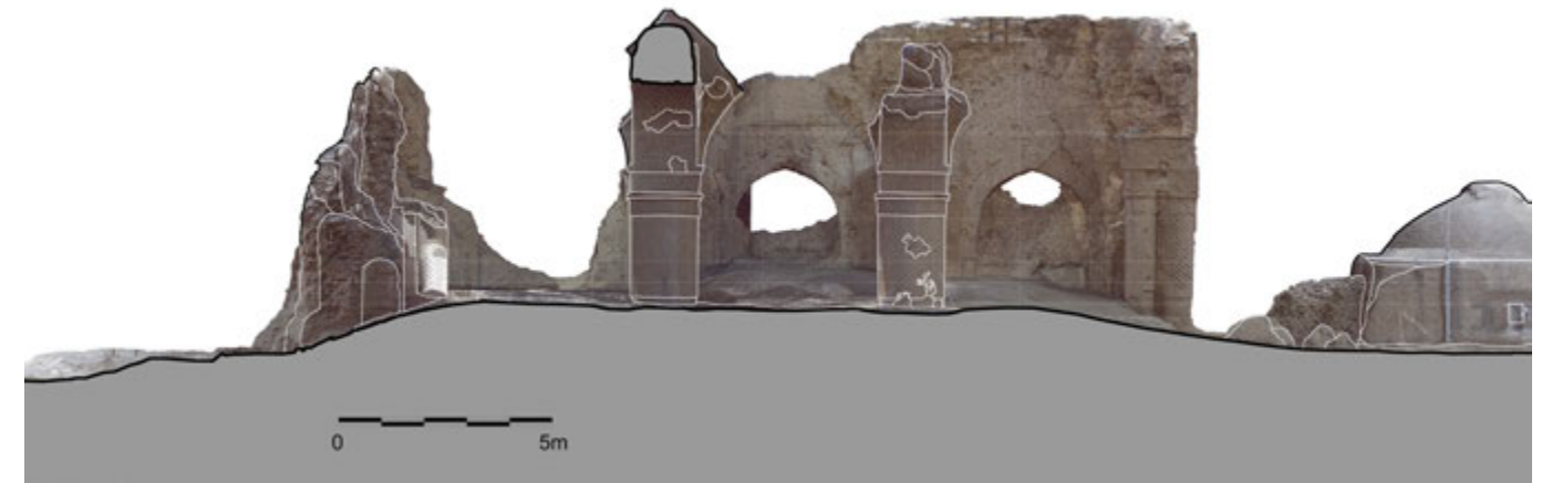
4. Longitudinal section (facing north), through the centre of the mosque and the mihrab (left), showing the internal elevations of free-standing columns 7 and 11.
